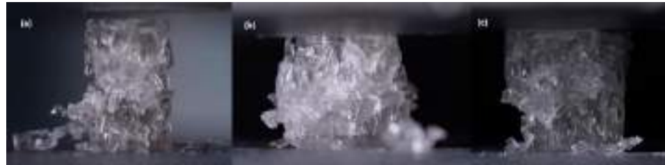
Figure 11. Failure mode of homogeneous elongated Voronoi structure. (a) Fracture prediction starts; (b) collapse; (c) fracture propagation.
