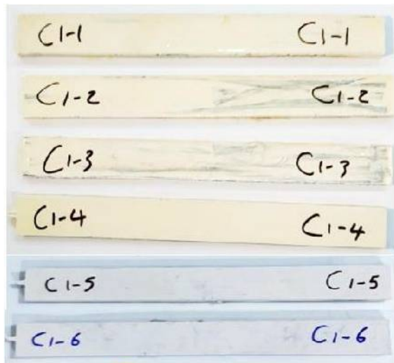
Fig. 7. Samples tested in flexural.
