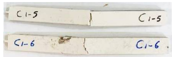
Fig. 12. Samples tested in flexural
