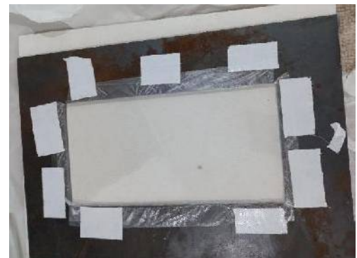
Figure (5): The front pf the mold is cased inside for ease emerging and using sticks for adopting.
