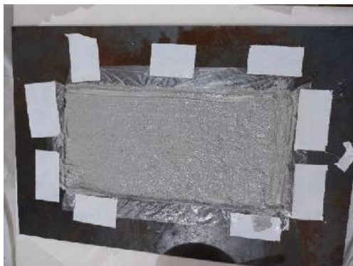
Figure (6): First layer epoxy resin
