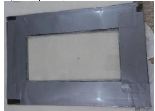
Figure (4): Preparing the mold by using on backside a limp paper and adopting a stick for all sides.
