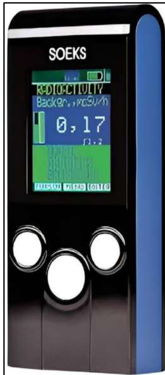
Fig.2. SOEKS 01M radiation detector (Germany Secondary Standard Dosimetry Laboratory Calibrated G.M. detector).
