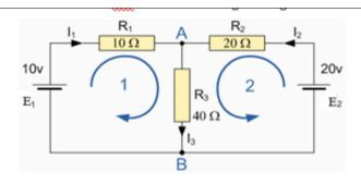
At node A:  $I_1 + I_2 = I_3$ At node B:  $I_3 = I_1 + I_2$
