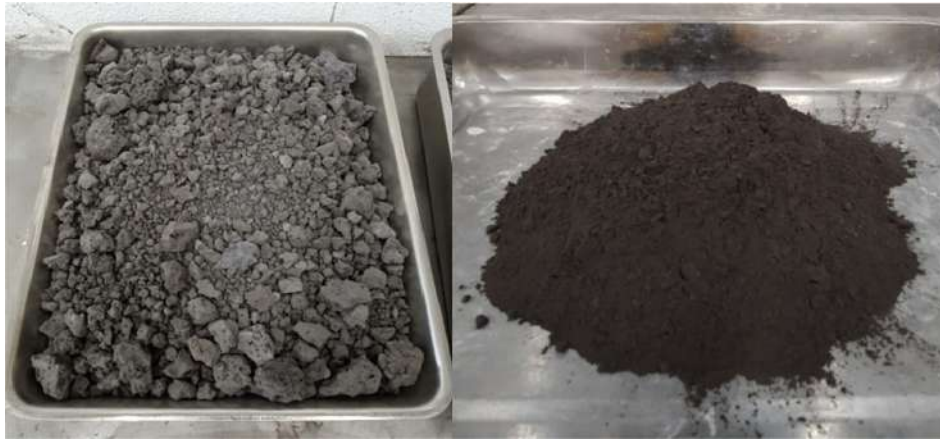
Fig. 3. EAFS as-received (left) and after milling to the required size for use as a precursor in concrete (right).
