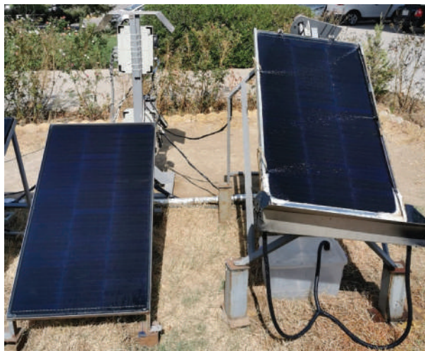
Figure 2. PV with and without cooling module rig.
