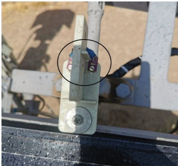
Figure 3. Tracking ambient light intensity sensors.
