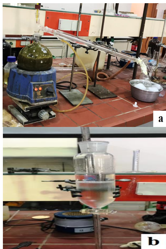
Fig.1: Hydro-distillation apparatus (a) and recovering the essential oil from distillation water using diethyl ether (b)
