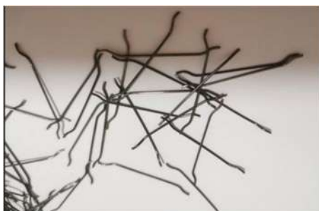
Figure 4. Double-hooked end steel fibers (DHE-SFs).
