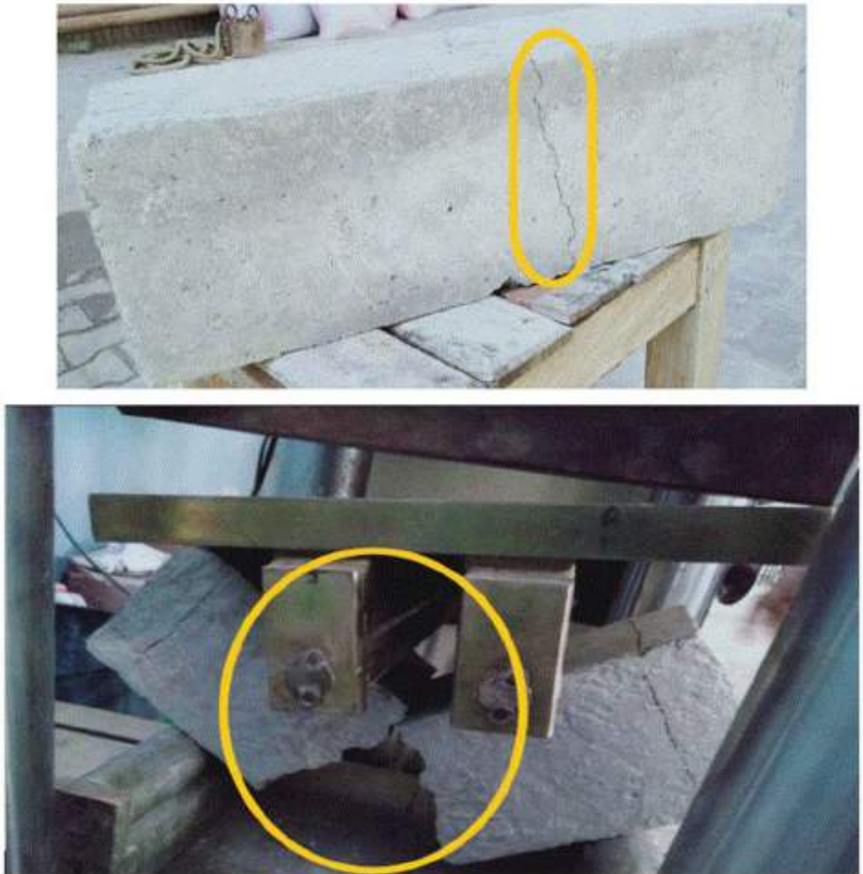
Fig 15. Failure patterns of UHPGPC under flexural load; (a) M1-GW-15, (b) M3-WRP-15.
