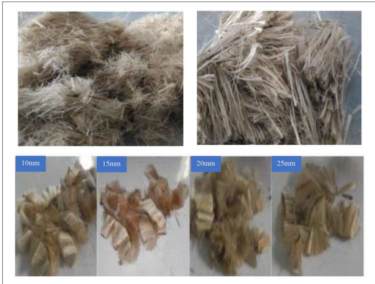
Figure 1. Jute fibers of different lengths used in concrete. 49,50
