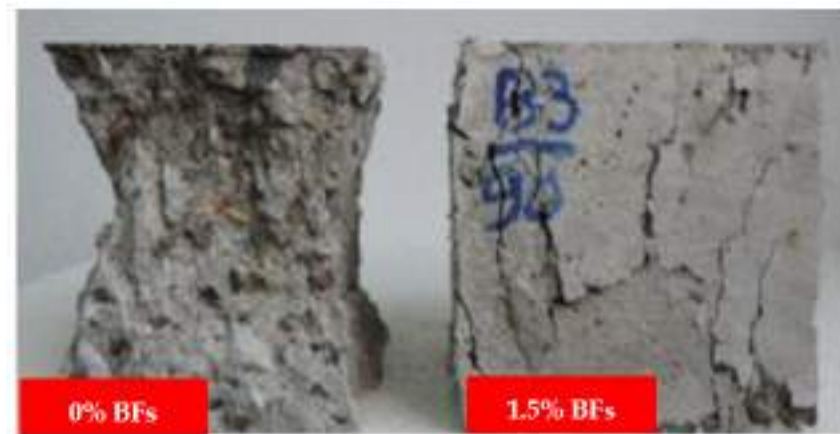
Figure 7. Compressive Failure Modes [50] with Elsevier permission.
