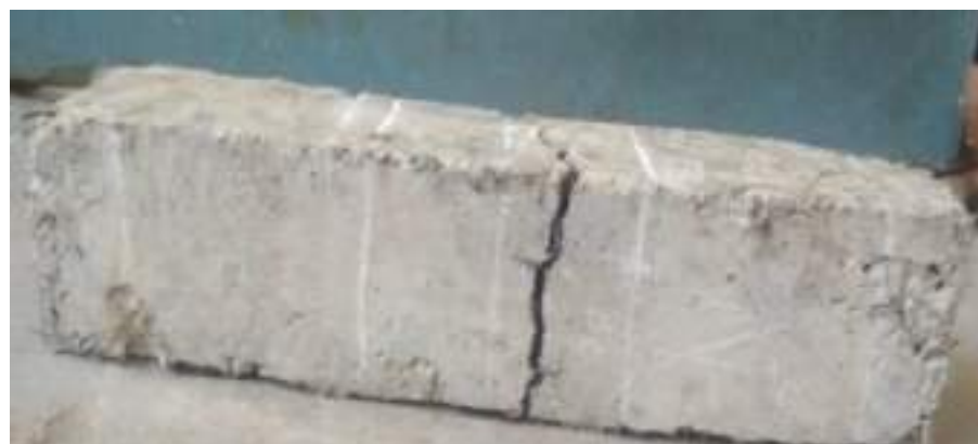
Figure 13. Failure of 1.5% Basalt Fiber Reinforced Concrete [50] with permission of Elsevier.
