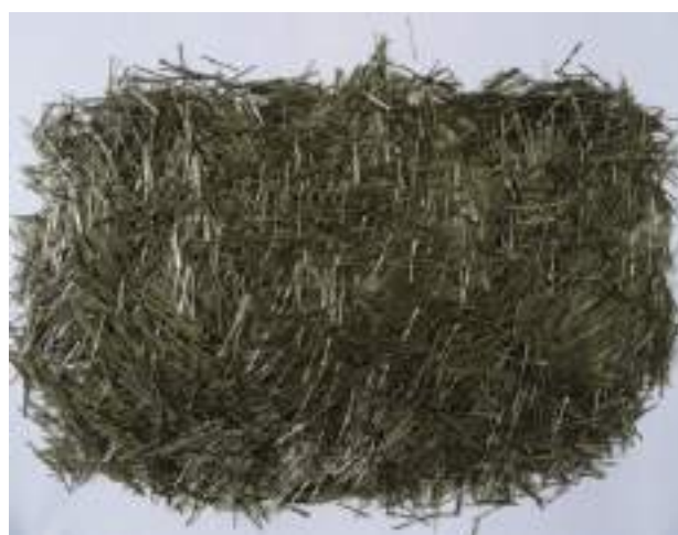
Figure 2. Basalt Fibers [30] with Elsevier permission.
