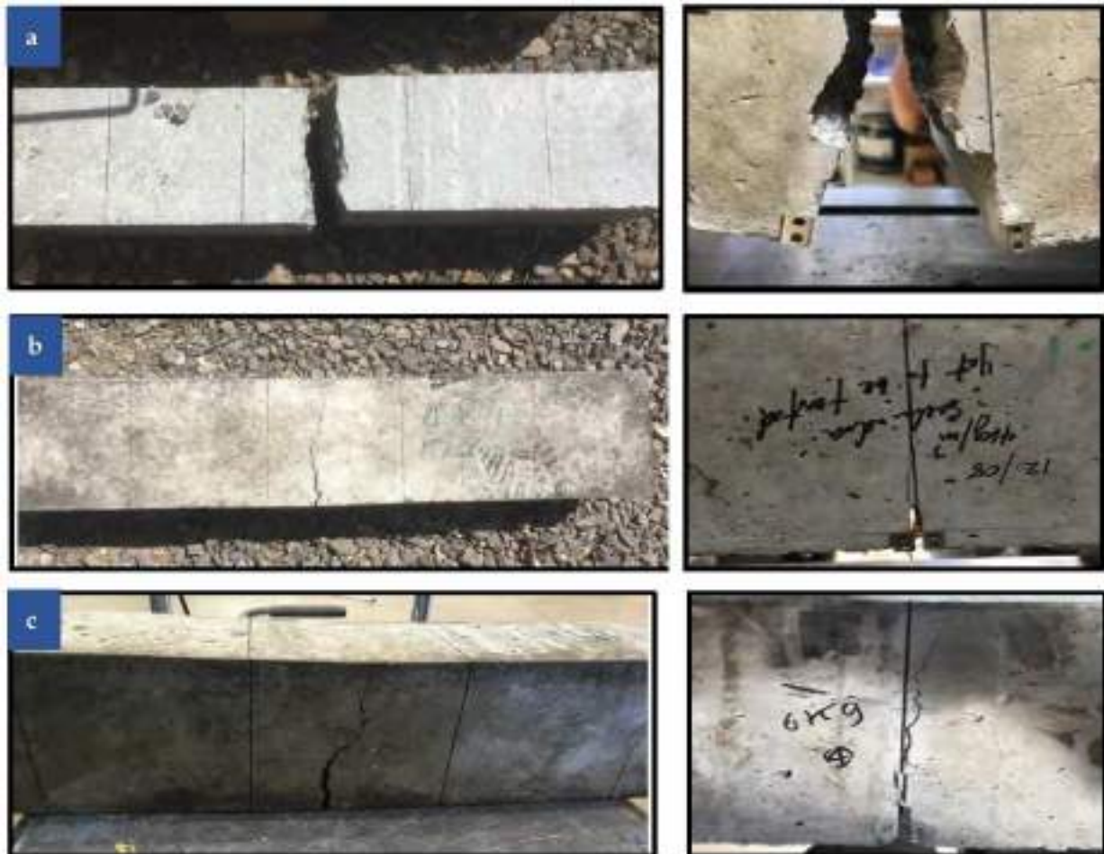
Figure 10. Flexural Failure modes: (a) 0%, (b) 4 \text{ kg/m}^3 and (c) 6 \text{ kg/m}^3 [82]; open access source.
