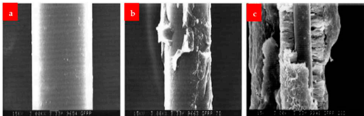
Figure 16. GF (a) normal, (b) 7 days under NaOH and (c) 28 days under NaOH [30].
