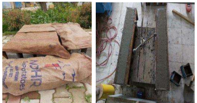
Figure (2) casting and curing of the specimens
