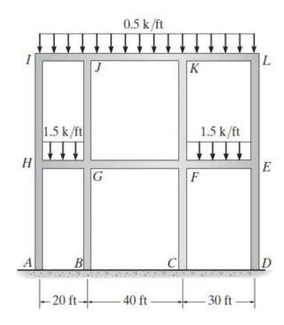
Q4/ Determine the reactions at the supports, then draw the moment diagram. Assume A is a pin and B and C are rollers. El is constant. Use force method. (20 Marks)
