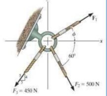
Resultant Force: Summing the force components algebraically along the x and y axes,
