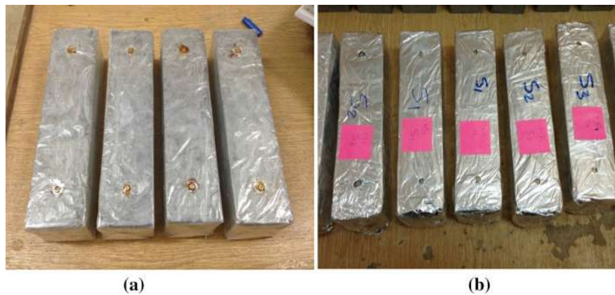
Fig. 2 Preparing the specimens for autogenous deformation a Pre-sealing of specimens with two layers of plastic sheets b Final sealing of the specimens with a layer of aluminum foil
