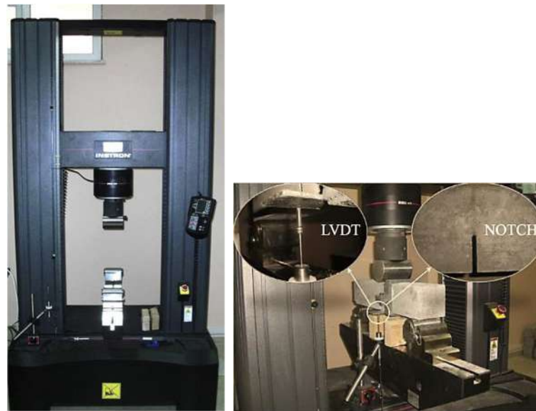
Figure 2. Three-point bending testing machine and test specimen [25] used for calculation of modulus of rupture.
