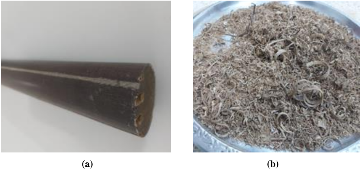
Figure 1 (a) Mica fiber (Phenolic Cotton Laminated Rod), (b) Mica fiber after grinding by a wood wool machine.
