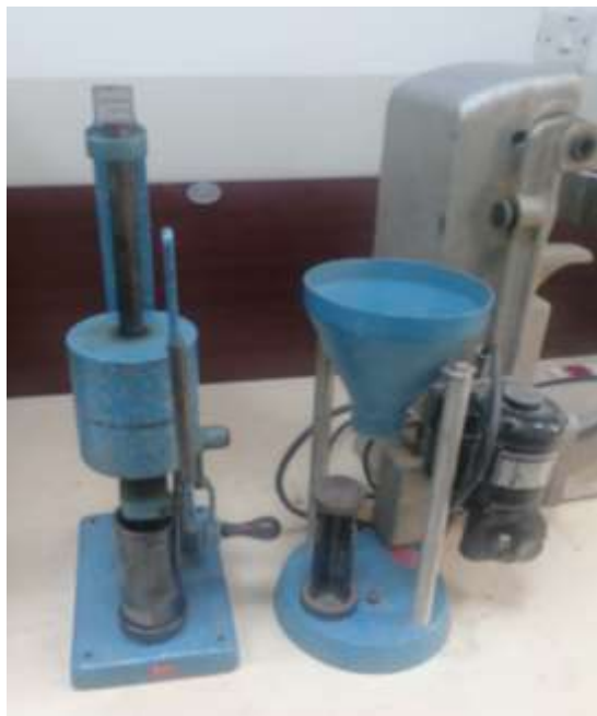
Fig. 2. Manual compactor instrument (Metric standard sand rammer).
