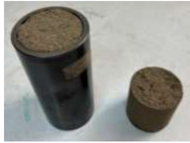
Fig. 3. A standard sample of the sand mould (Strip block and specimen test piece).
