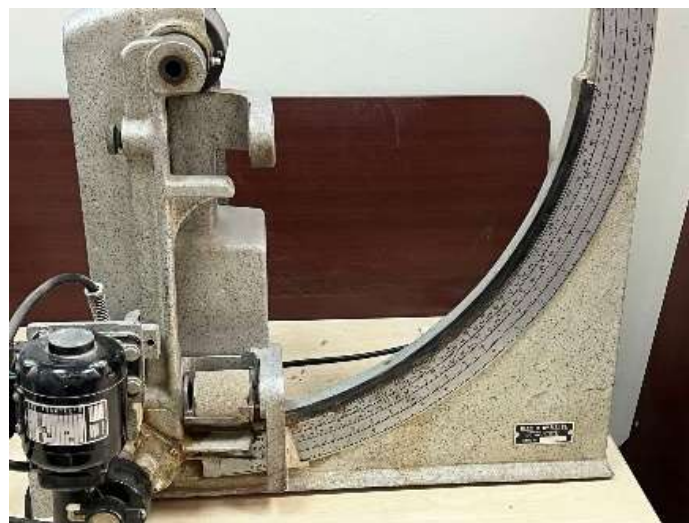
Fig. 5. universal sand strength machine.
