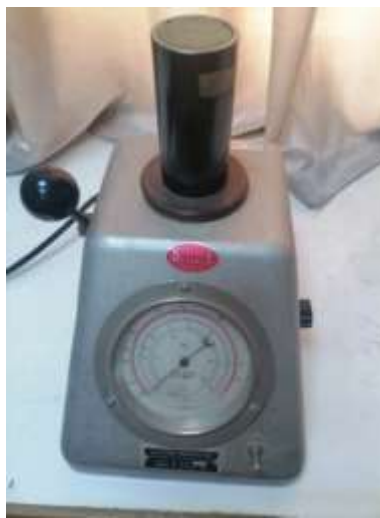
Fig. 4. Electric permeability meter apparatus.
