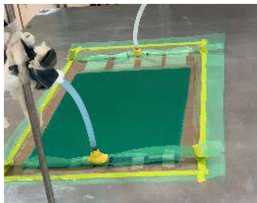
Fig.( 2):- Vacuum bagging technique
