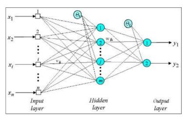
Fig 1: Back propagation neural network
