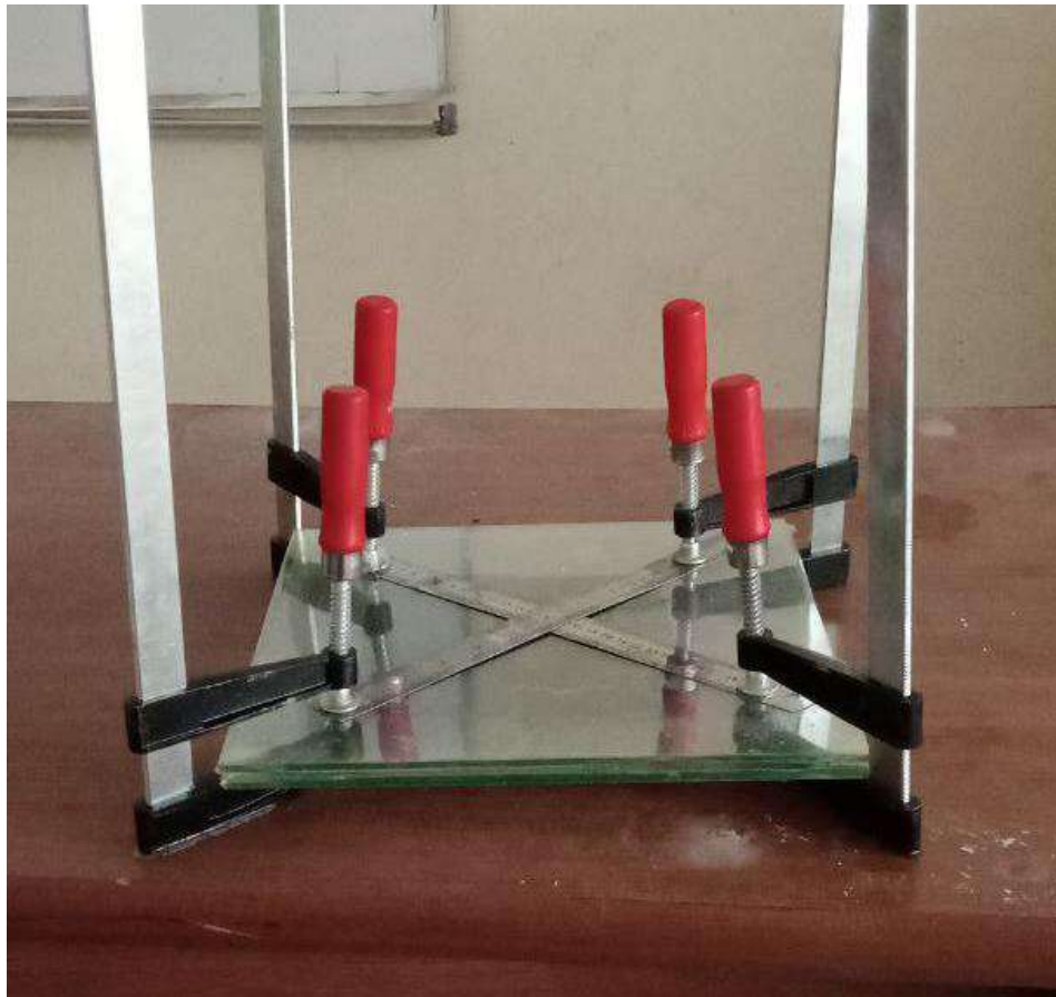
Fig. 3. Composite plate preparation by hand layup and prepreg method, source: Author's own creation.
