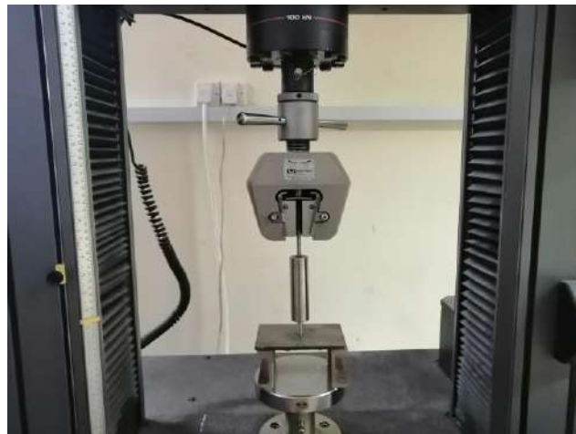
Fig. 5. Blister test sample under the tensile testing machine, source: Author's own creation.
