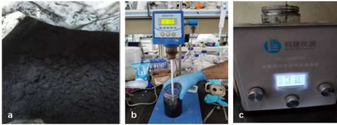
Fig. 1. Mix epoxy with MWCNTs: a) MWCNTs, b) digital mixer, c) ultra-sonication
