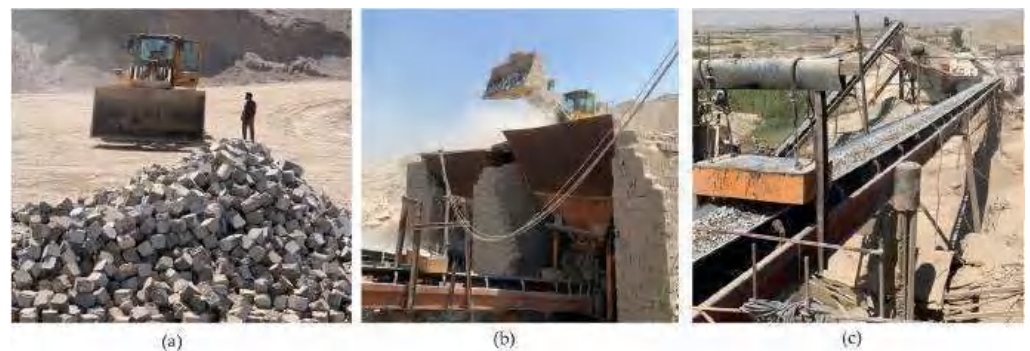
Figure 1. Production of recycled coarse aggregate: (a) waste concrete; (b) crusher; (c) recycled aggregate.
