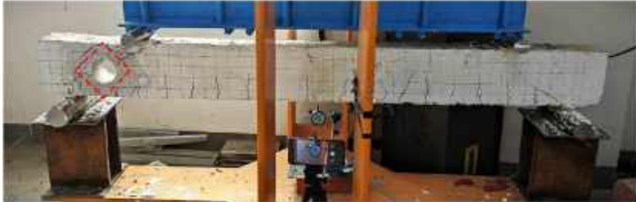
f) The patterns of crack observed and the failure mode for specimen DBLSD10.
