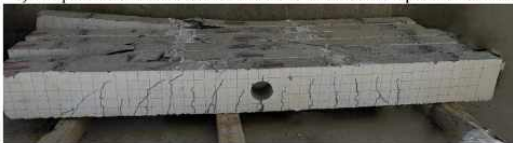
c) The patterns of crack observed and the failure mode for specimen SBLF.
