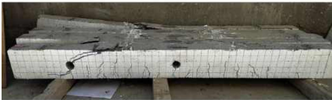
f) The patterns of crack observed and the failure mode for specimen SBSSF
