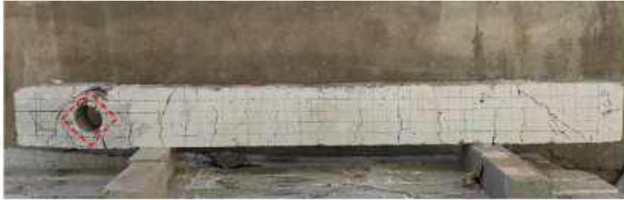
e) The patterns of crack observed and the failure mode for specimen DBLSD8.
