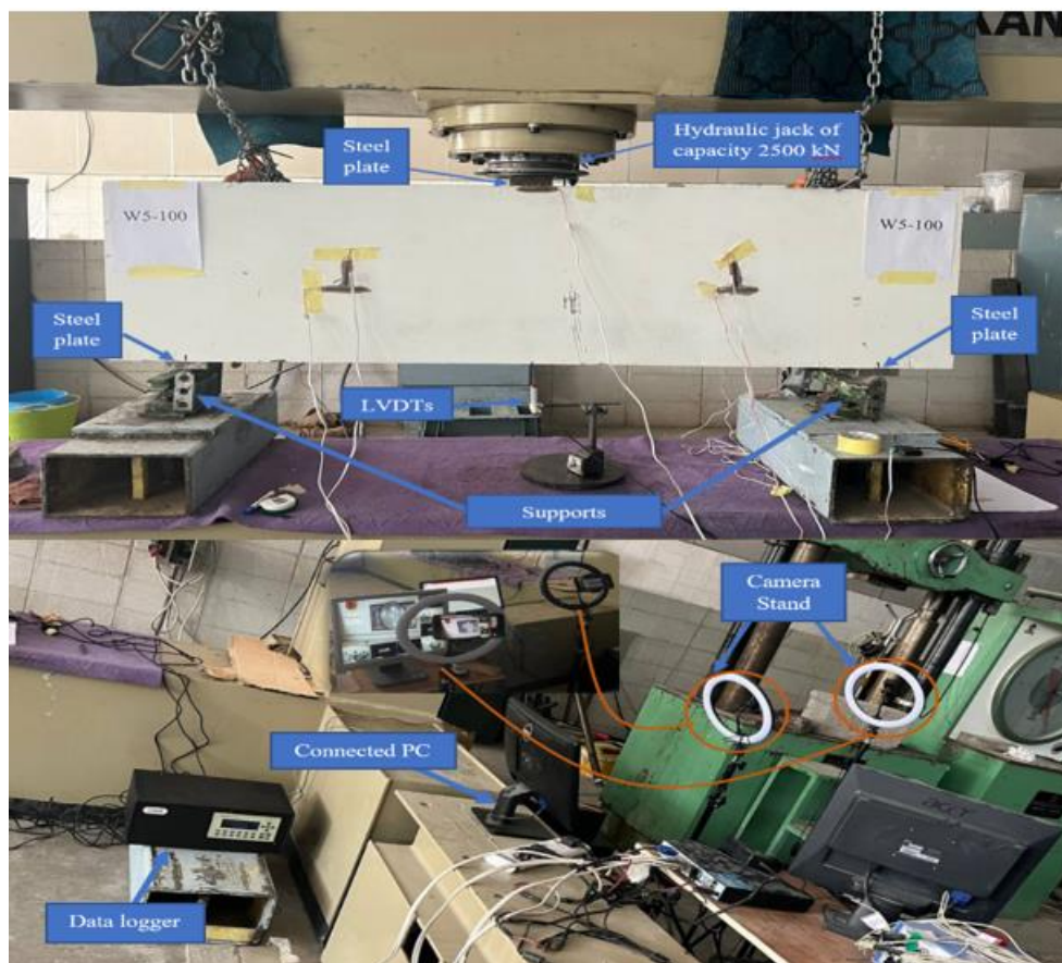
Figure 3: Testing configuration of beam specimens
