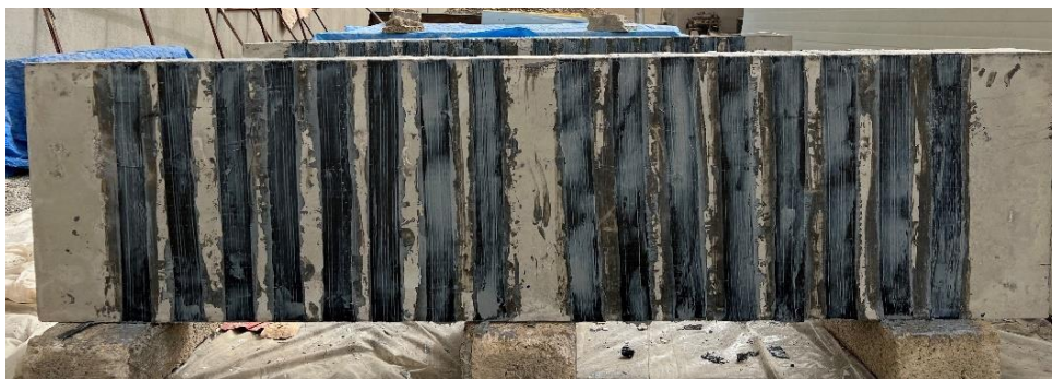
f) Final shape after CFRP strips strengthening from one side.
