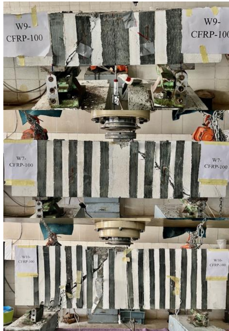
Figure 5: Crack patterns for beams of G2 at ultimate loads
