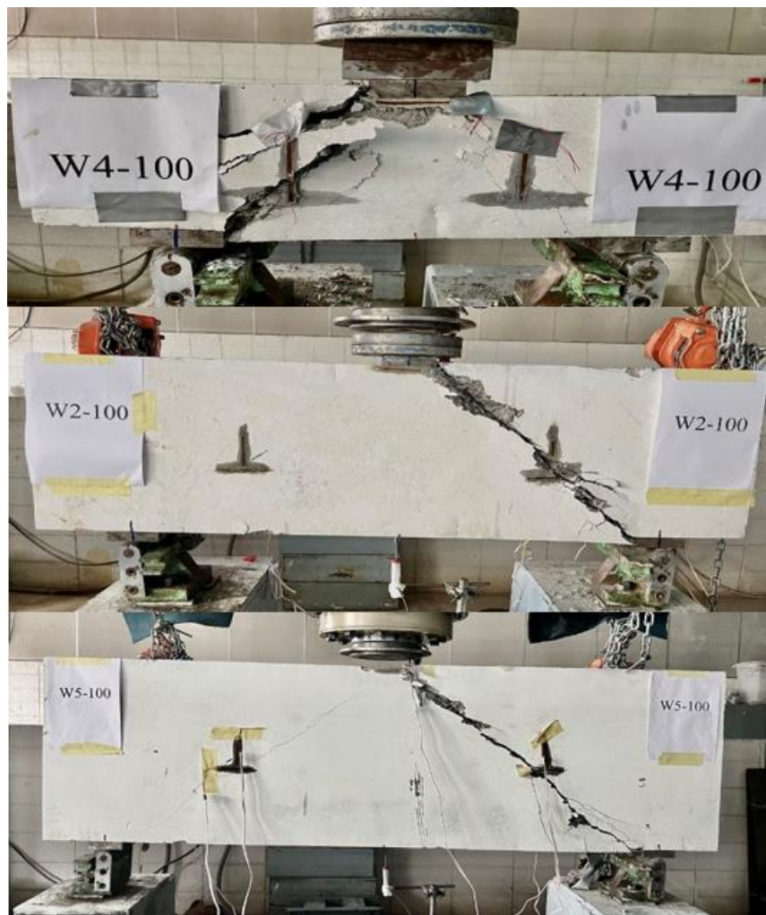
Figure 4: Crack patterns for beams of G1 at ultimate loads
