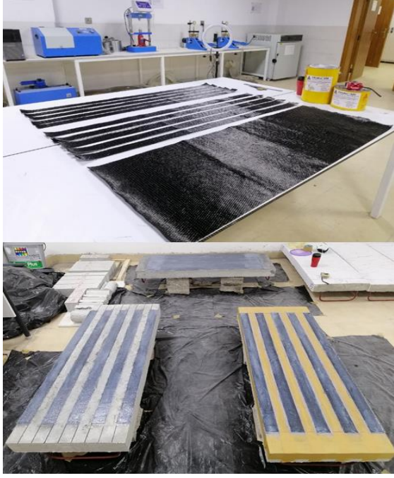
Figure 4. Sika wrap 300C and Sikadur 330 & strengthened specimens Instrumentation and testing procedure
