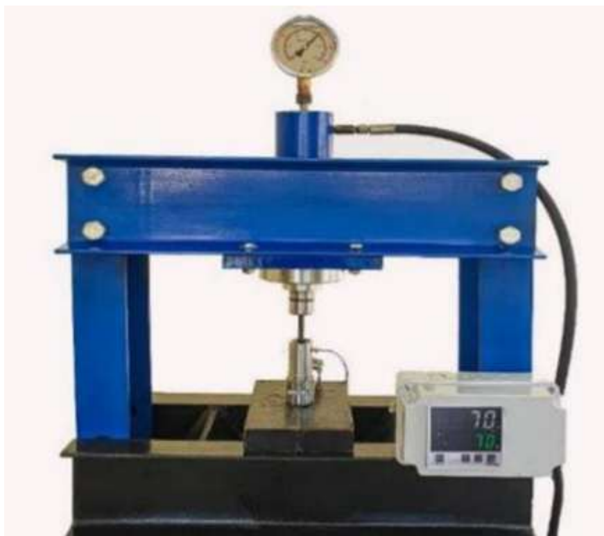
Figure 2: pellet extruding die in a manual hydraulic press with control box
