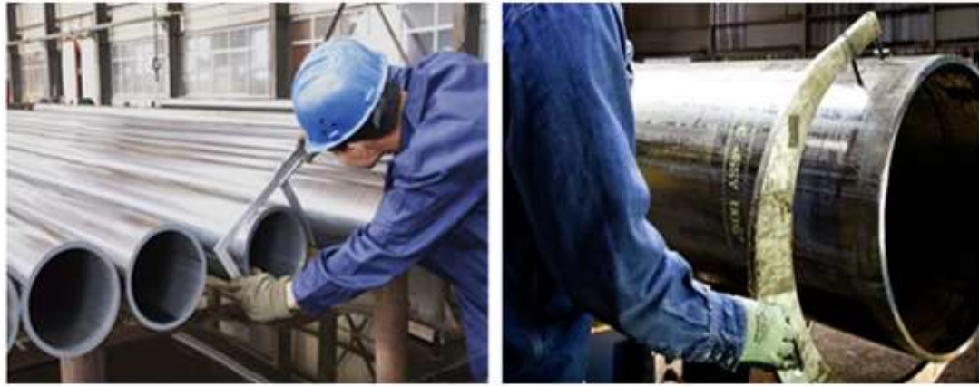
The figures show the inspection process of diameter of manufactured steel pipes in an industry factory
