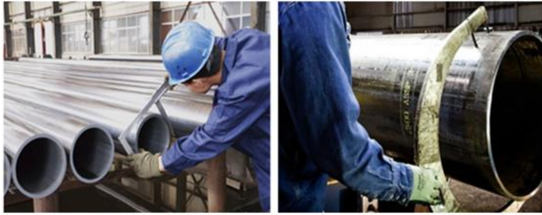
The figures show the inspection process of diameter of manufactured steel pipes in an industry factory
